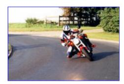
The bike is light, with the weight cenetered low. This, and its small physical size. means it's an easy bike to manage even if your body isn't held as far off the ground by your legs as you'd like. For this reason, and the low 770mm (30.3 in) seat height, it would make an excellent choice for the *girls*. Wheeling it in and out of the garage is a doddle, aided by the upright bars and low center of gravity.
