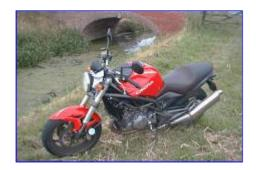
Power is no good without control, or so the saying goes. Lucky, then, that Cagiva wrapped the motor in a Ducati-inspired (or is it Rickman inspired?) steel-tube, trellis-type chassis. The inverted 43mm Marzocchi front forks did feel a little hard in bumpier corners which led to a tendency for the Raptor to shake its head exiting corners on less than smooth pavement. This front-end nervousness is exaggerated by the handlebars
