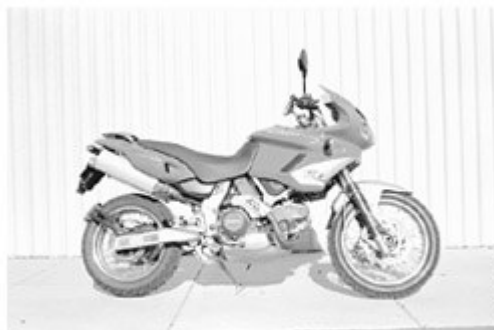
Cagiva's dual-sport is powered by a fuel-injected Ducati V-Twin.
