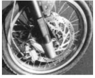
The brakes are excellent Nissin twin-piston, single-action types, like those that came on the CBR600F3. They have good power and feel, but the block-pattern tires tend to limit stopping distances.
