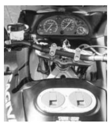
Twin fillers allow the fuel nozzle deep into the tank, but take extra time to unlock. A small diameter crossover tube allows them to drain evenly, however. Instruments are easy to read except for the red mph markings around the kph speedo. Both left and right turn signal indicators flash together. Satin black paint looks military, which is cool, and prevents annoving reflections.
